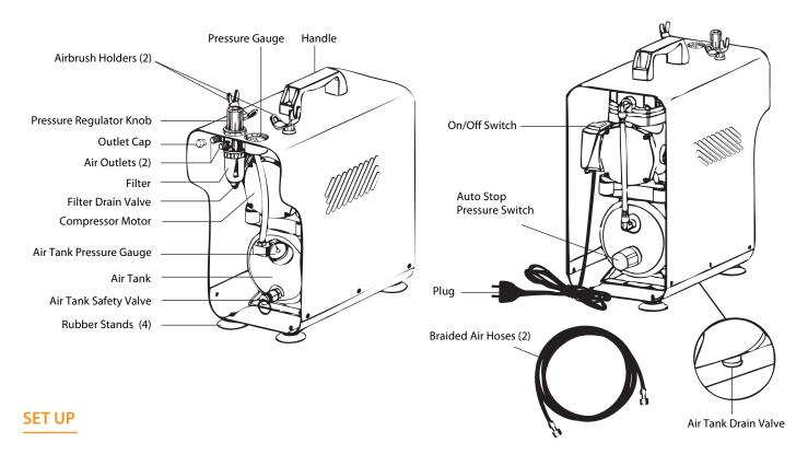
1. Screw the 1st Braided Air Hose onto the airbrush and Air Outlet.
