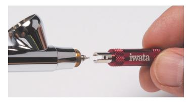
Removing or tightening a screw-on nozzle is a routine maintenance task that can sometimes feel difficult to do, mainly because they are small and hard to hold onto. The Iwata Nozzle Wrench makes it a lot easier. The nozzle seats within the end of the nozzle wrench tool and allows you to easily hold the nozzle as it is being aligned into the threads of the airbrush body.
